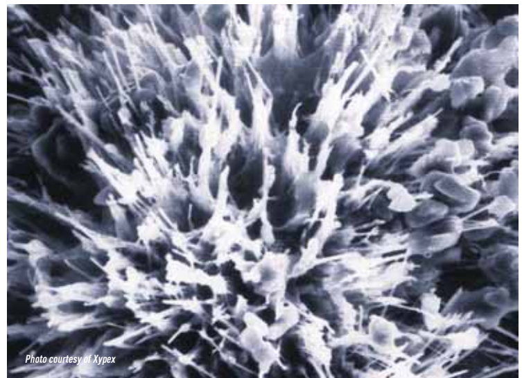
Scanning electron microscope (SEM) view of a concrete pore filled with multiplicative crystalline formation, initial stages.
